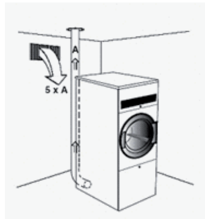
Figure 5. Relationship between intake and evacuation air.
